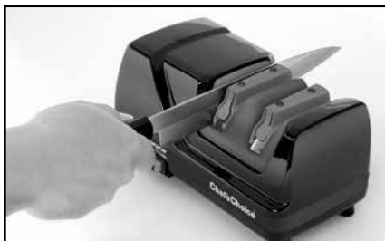
Figure 5. Traditional (sushi) knife in left slot of Stage 2. Figure 6. Traditional (sushi) knife in left slot of Stage 1.
