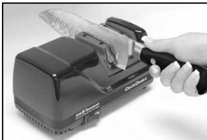
Figure 3. Santoku knife in right slot of Stage 1.
