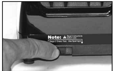
Figure 11. Cleaning the polishing disks (see text).
