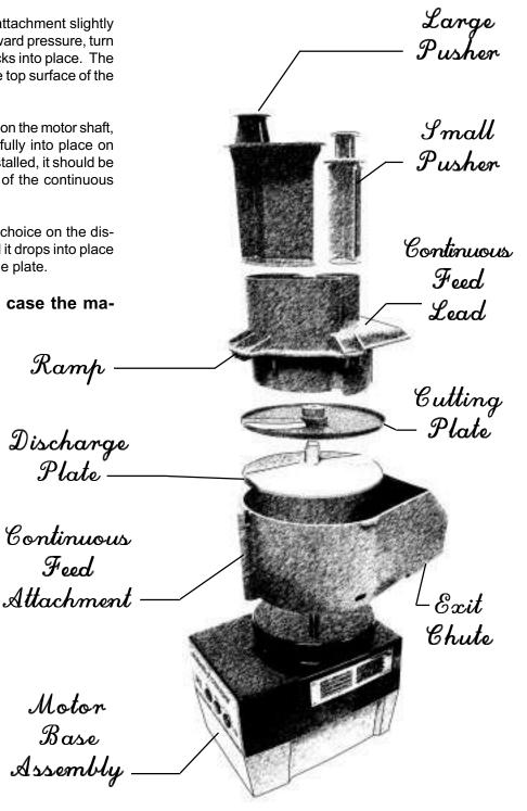
The continuous feed lead, with the pushers in place, provides protection from the cutting plate. When the lead is turned to it's closed position with the ramp in place over the pin, a safety switch is activated, and the machine can be turned on and off by use of the push buttons. If the lead is not in the closed position, the buttons will not function.
