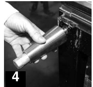
4 Thread leg into cabinet bottom frame rail.
