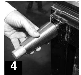
4 Thread leg into cabinet bottom frame rail.
